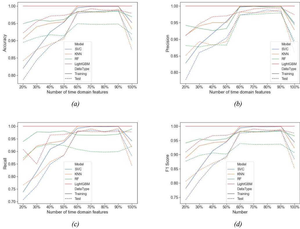
Figure 8 – Results of SVC, KNN, RF and LightGBM when different percentages of features are selected as inputs after ranking the time-domain features with significance in order of random forest importance
