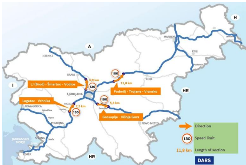
Figure 4 – Sectional speed control on Slovenian motorways; Source: DARS
