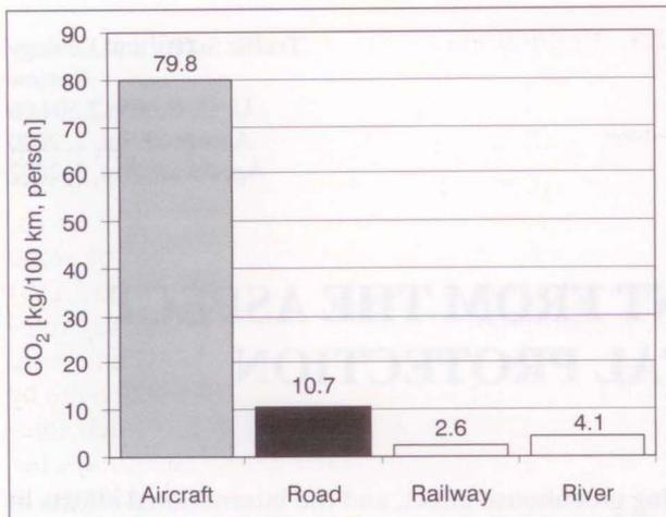
Figure 2 - Specific CO<sub>2</sub> emission of individual branches in cargo transport
