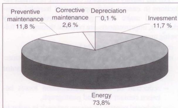
Figure 3 - Share of individual LCC of a cargo locomotive
