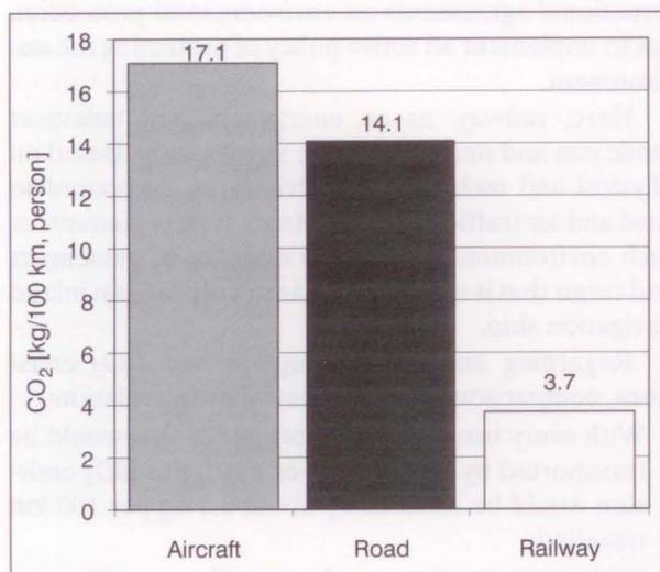
Figure 1 - Specific CO<sub>2</sub> emission of individual branches in passenger transport
