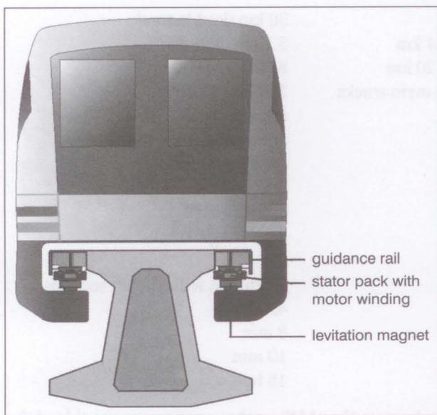
Figure 5 - Cross section
