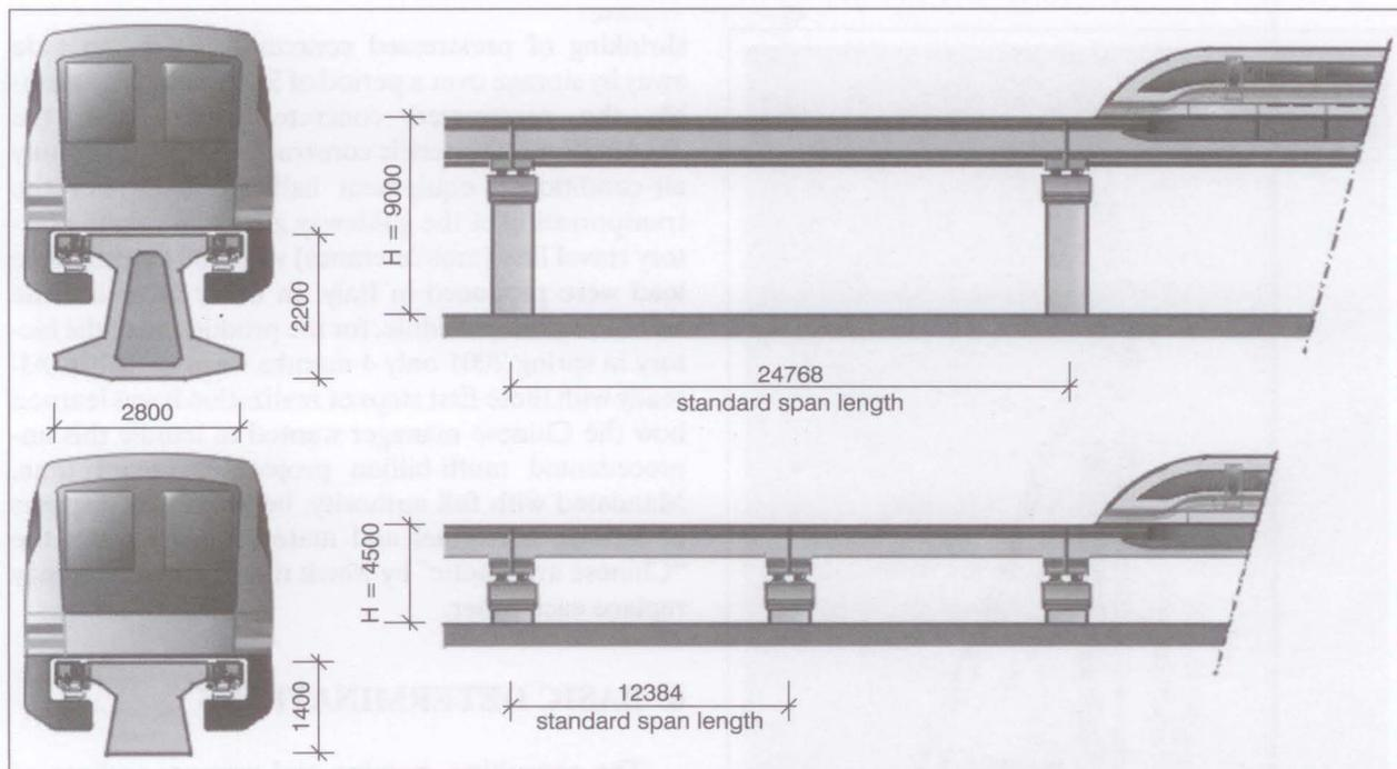
Figure 7 - Hybrid guideway girders of the Shanghai project
