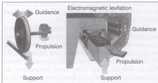
Figure 2 - Levitation and propulsion
