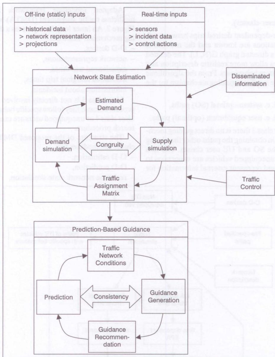
Figure 1 - Structure and processes in anticipatory real-time guidance system
