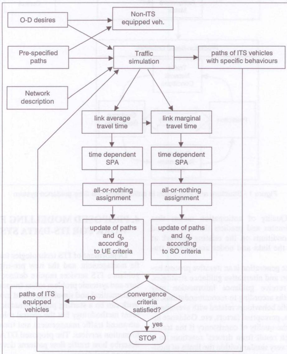
Figure 2 - Modelling framework for dynamic traffic assignment in ITS environment
