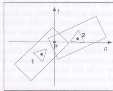
Figure 2 - Oblique collision used in the impulse model
