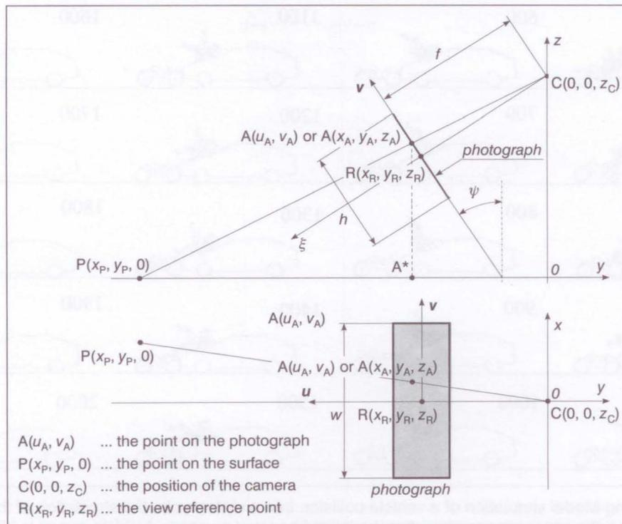
Figure 7 - Transformation of a photograph point A into a surface point P
