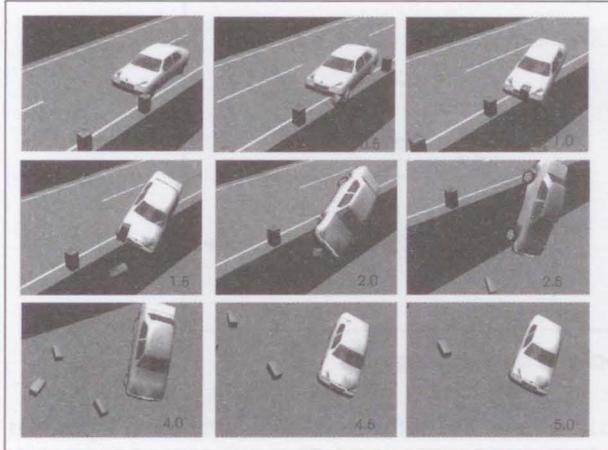
Plate 1 - PC-Crash simulation of a collision of a vehicle into side-road barrier-type stone and the initial motion of a vehicle over side-scarp at the speed of 37 km/h.
