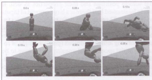
Plate 3 - PC-Crash simulation of a pedestrian's rebound from a car hood shown from the driver's perspective
