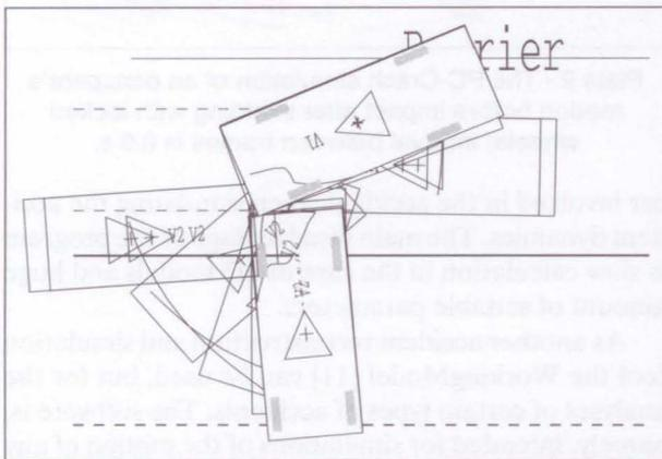
Figure 6 - The results of m-smac computer simulation of a two-vehicle collision; individual positions of the vehicles are plotted in 0.25 s intervals.
