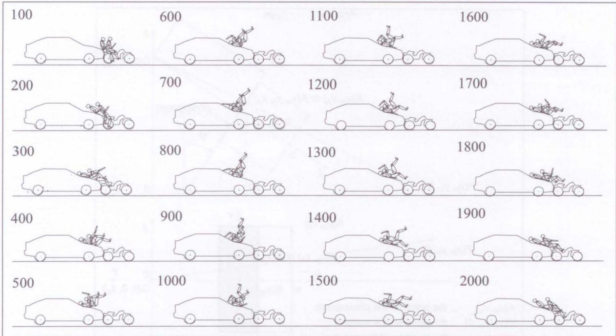
Plate 5 - Working-Model simulation of a vehicle collision into a motorcycle, the simulation of the motorcycle driver and the passenger motion after the initial impact of a vehicle (vehicle speed is 72 km/h, while the motorcycle speed is 36 km/h; intervals between frames are in  $\mu\text{s}$ )
