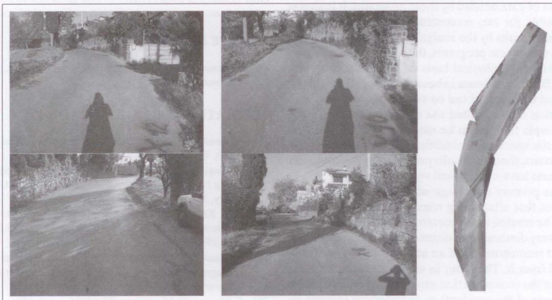
Plate 6 - Original photos of an accident scene and rectified picture of a blind curve (right); the rectified picture is composed from three independently rectified original photos
