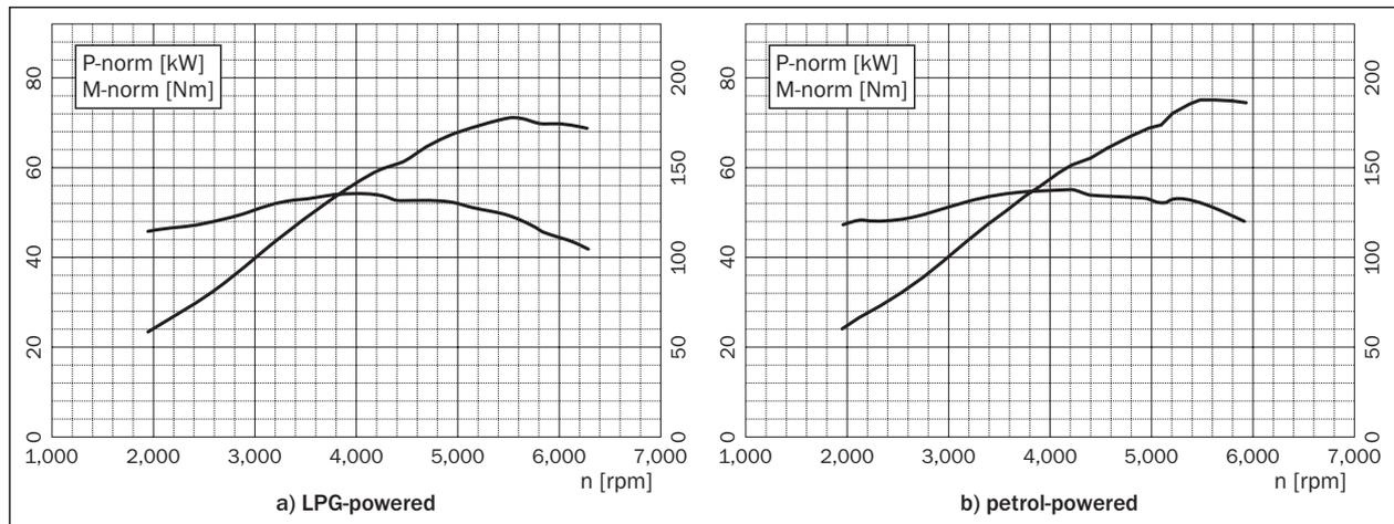
Figure 7 - Diagram of moment and power of vehicle with gas installations at the end of testing (40,464km)
