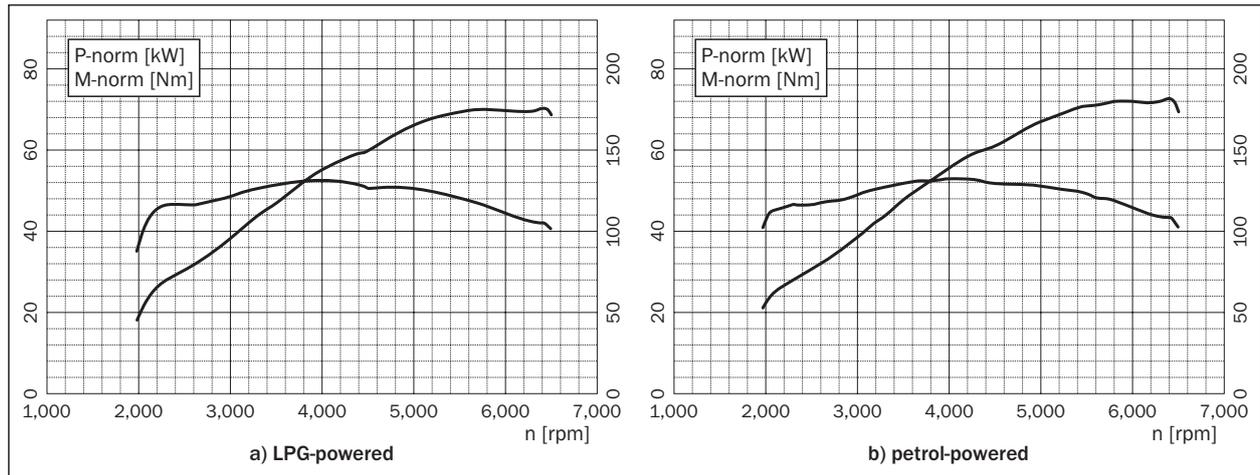
Figure 6 - Diagram of moment and power of vehicle with gas installations at the beginning of testing
