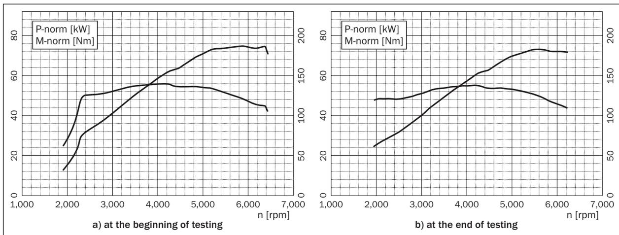
Figure 5 - Moment and power diagram of petrol-powered vehicle
