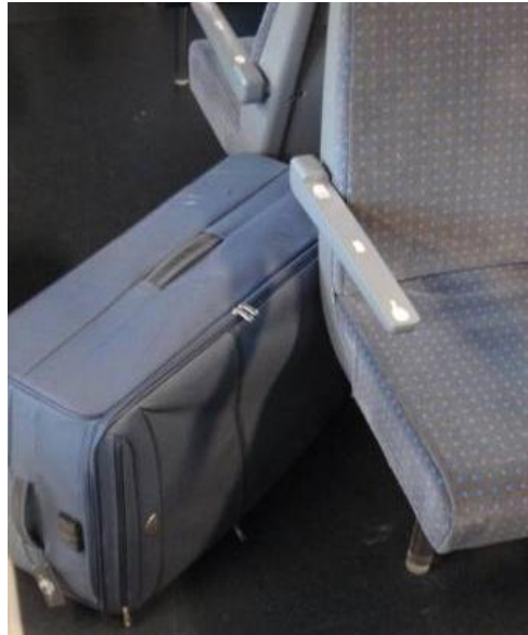
Figure 7 – Areas behind the seat backrests, too little space for threading due to the narrow aisle width (photo: R ger Bernhard)
