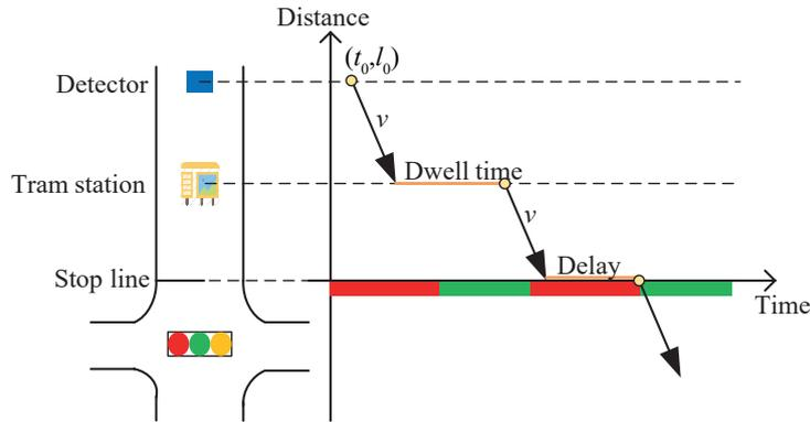
Figure 2 – Tram operation process
