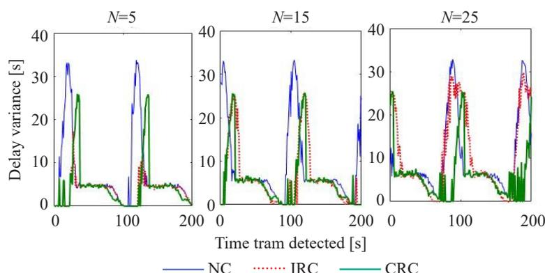
Figure 12 – Tram delay variance when station serves multiple lines
