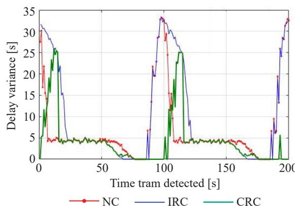
Figure 9 – Tram delay variance when station serves a single line
