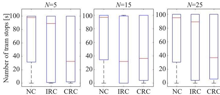
Figure 13 – Number of tram stops when a station serves multiple lines
