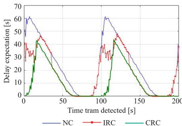
Figure 8 – Tram delay expectation when station serves a single line
