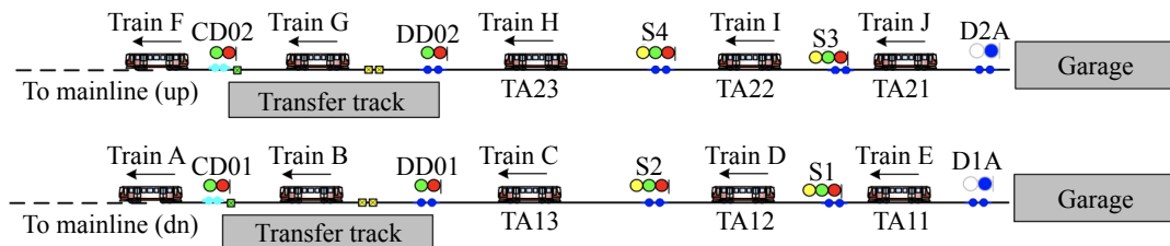
Figure 2 – Signalling system configuration and train tracking diagram in the depot after optimisation
