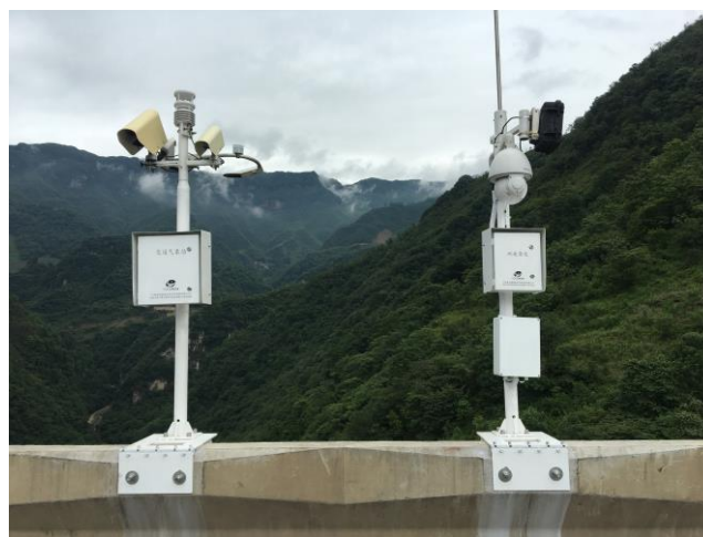
Figure 1 – Roadside traffic meteorological station located at Ma Zhao Expressway, Yunnan, China
