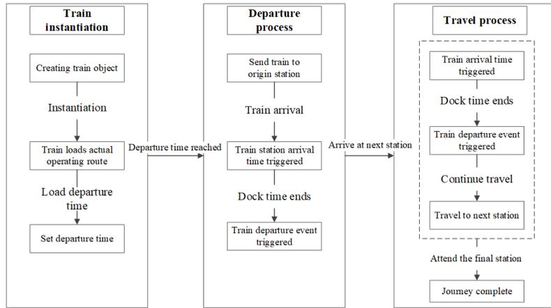
Figure 3 – Train simulation logic
