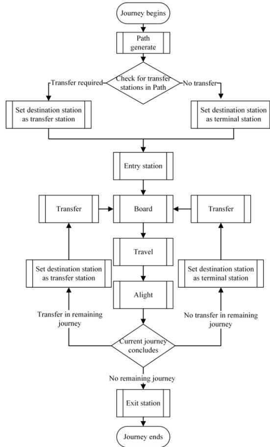
Figure 5 – Passenger travel simulation process
