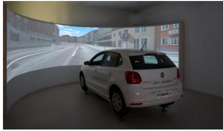
Figure 1 – Three degrees of freedom driving simulator
